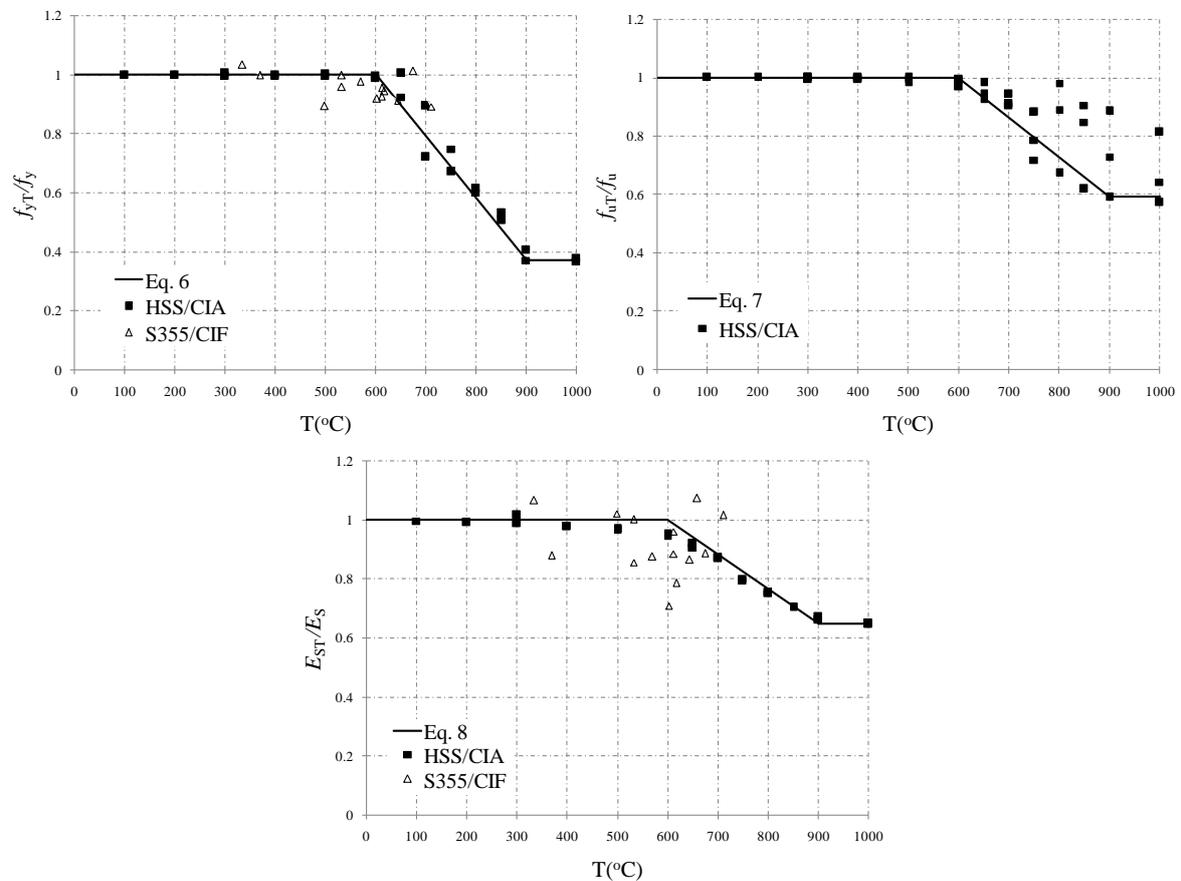
Fig. 5: Comparison of predicted residual factors for heat-treated steel
