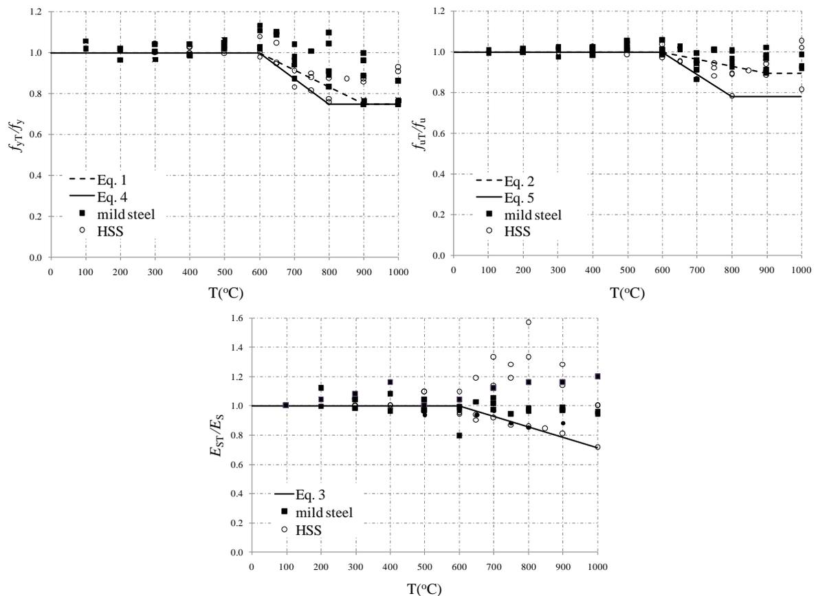
Fig. 4: Comparison of predicted residual factors  $f_{yT}/f_y$ ,  $f_{uT}/f_u$  and  $E_{sT}/E_s$  for hot-rolled steel
