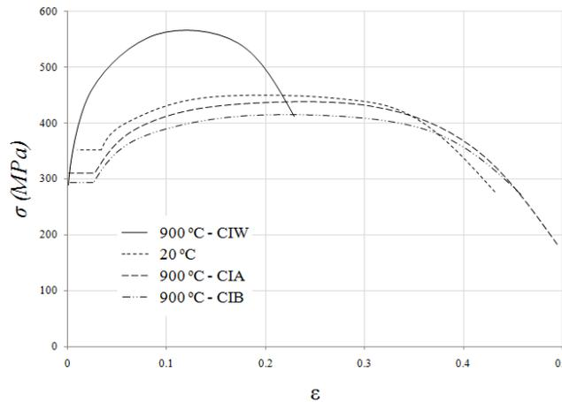
Fig. 2: Influence of different cooling methods on stress-strain curves [6]
