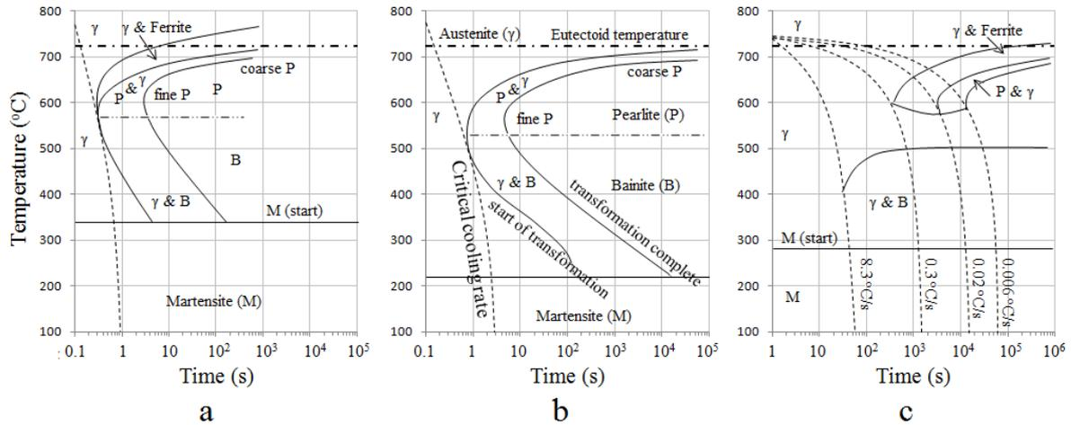
Fig. 1: Schematic diagrams illustrating isothermal curves (IT), critical cooling curves and resulting microstructures for (a) hypoeutectoid, (b) eutectoid and (c) alloy steel [12]
