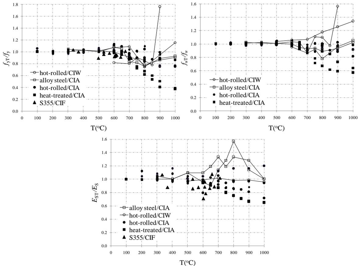
Fig. 3: Ratio of  $f_{yT}/f_y$ ,  $f_{uT}/f_u$  and  $E_{sT}/E_s$  as a function of temperature for structural steel
