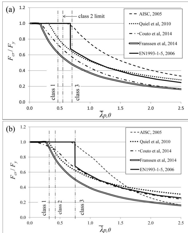
Fig. 1. Comparison of proposed design and code methods for capacity of slender plates at 500°C, (a) for stiffened plates (web) and (b) for unstiffened plates (flange).
