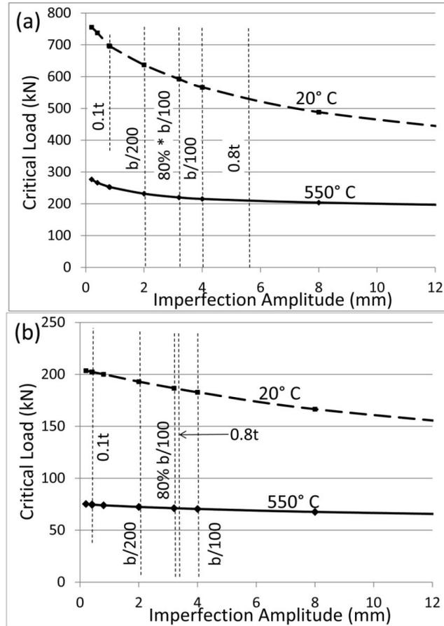
Fig. 2. Critical load vs local imperfection amplitude for four sides simply supported plates with (a)  $\lambda_{p,\theta}=1.0$  and (b)  $\lambda_{p,\theta}=2.0$  at 20 °C and 550 °C.
