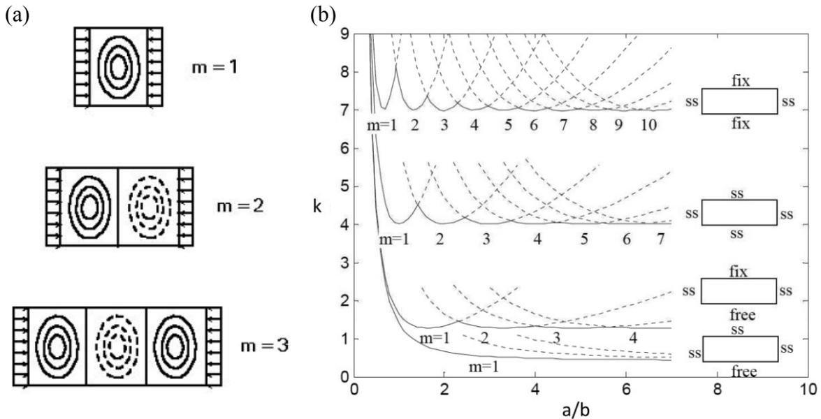
Figure 3. (a) Different buckling modes ( $m$  is the number of half-waves) for different  $a/b$  ratios of 4 sides simply supported plates and (b) buckling reduction factor for plates in compression as function of the shape of the plate  $a/b$ , the boundary conditions and the number of half-waves  $m$  [14].
