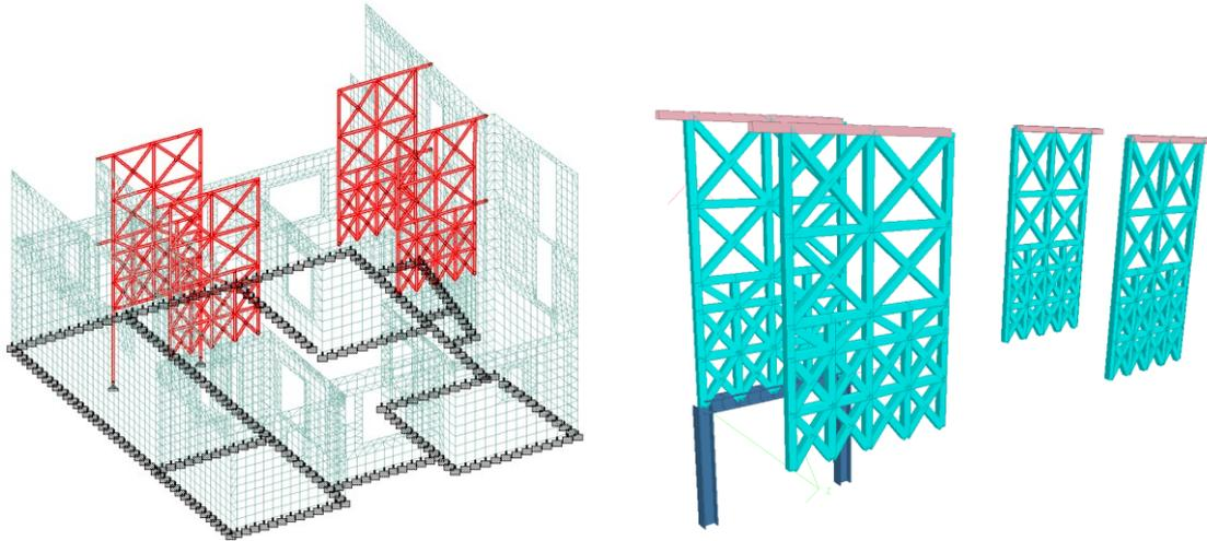
Figure 8: Strengthening proposal (addition of timber frames) for stiffness increase along the X direction.
