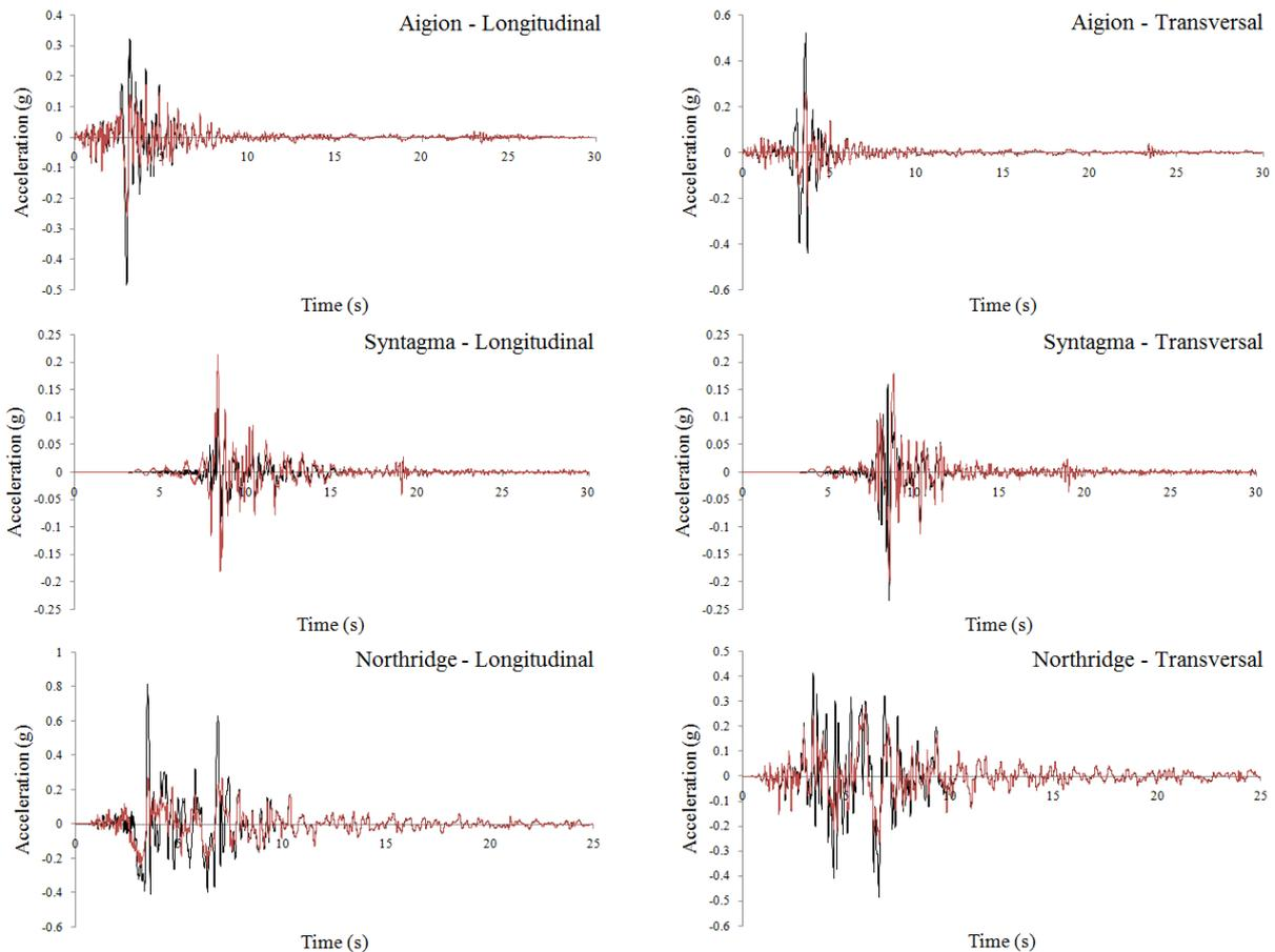
Figure 6: Time histories that were used for the dynamic analyses: original (black colored) and scaled (red colored) accelerations.
