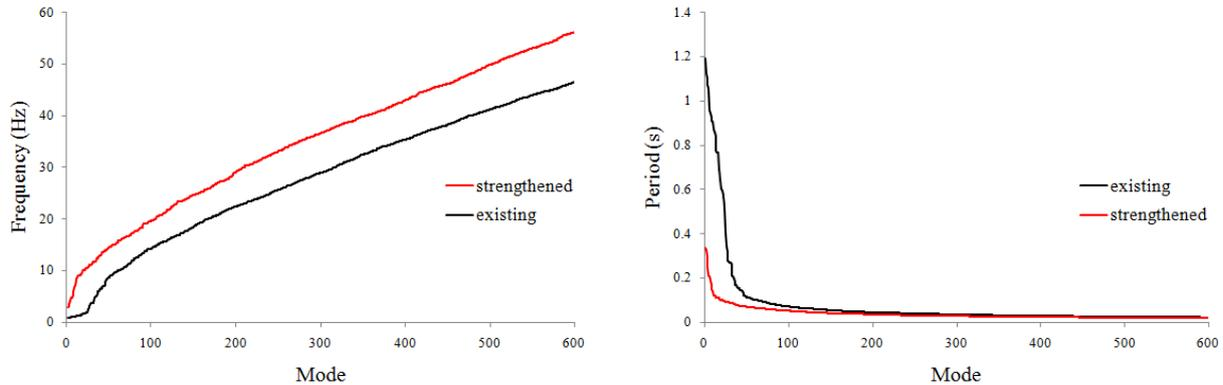
Figure 11: Comparison of mode frequencies between the existing and the retrofitted structure.
