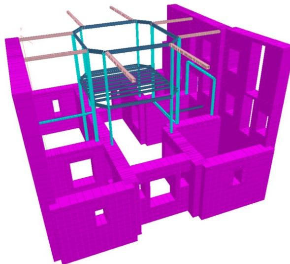
Figure 5: 3D view of the steel core and the masonry walls of the existing structure.
