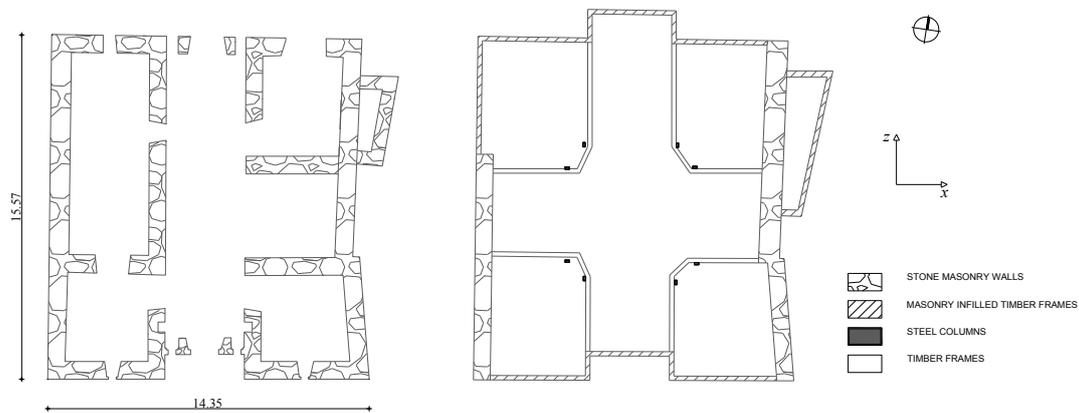
Figure 2: Plan of the ground floor (left) and 2nd floor (right).
