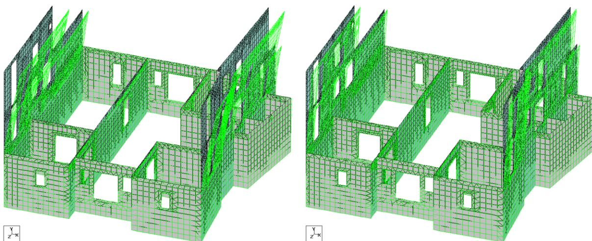
Figure 9: Stone masonry deformation under earthquake loading along the X direction , a) before and b) after strengthening.
