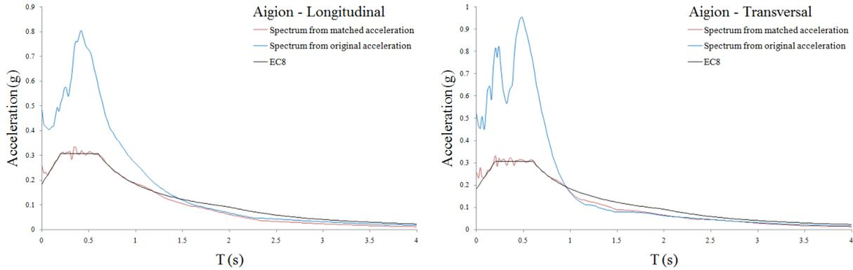
Figure 7: Response spectra derived from the Aigion earthquake (1995); comparison with the corresponding one from EC8 a) for longitudinal and b) for transverse direction.
