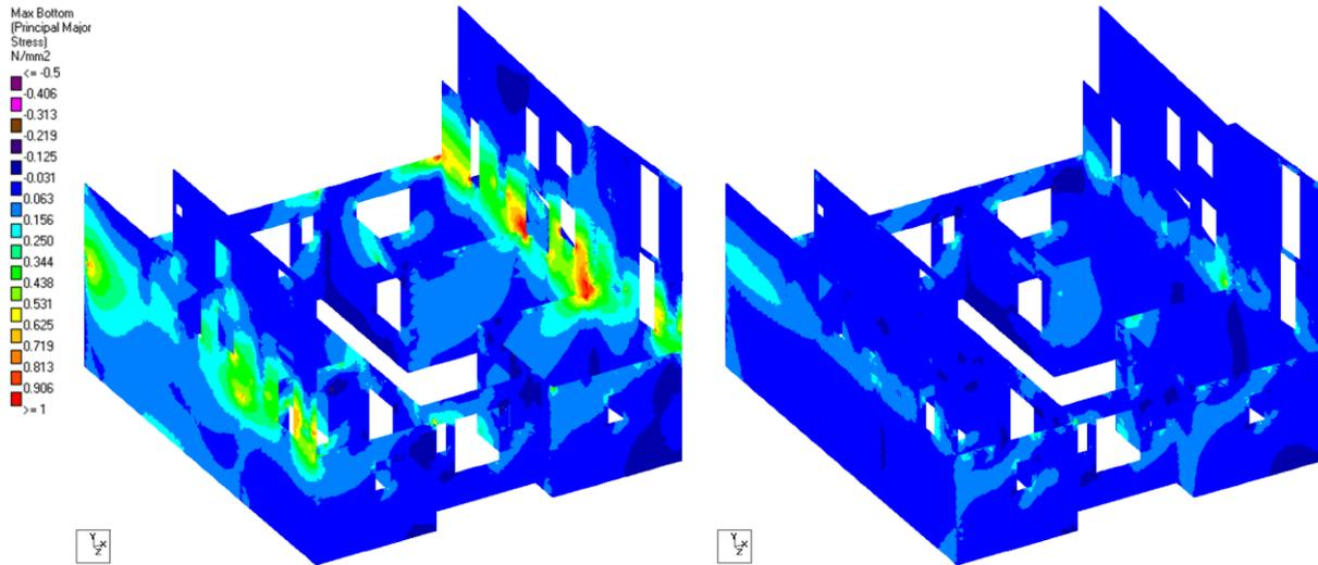
Figure 10: Major principal stress distribution under earthquake loading along the X direction, a) before and b) after strengthening.
