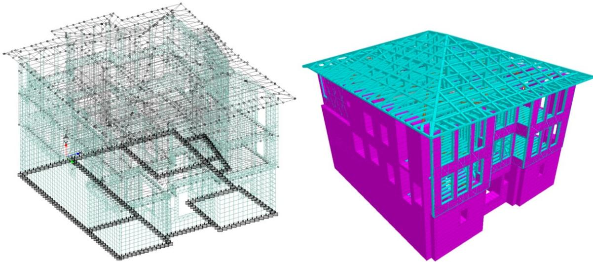
Figure 4: 3D view of the model used to simulate the structure.
