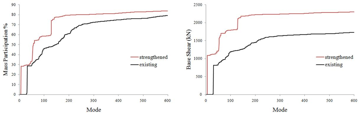
Figure 12: Comparison of base shear forces between the existing and the retrofitted structure.
