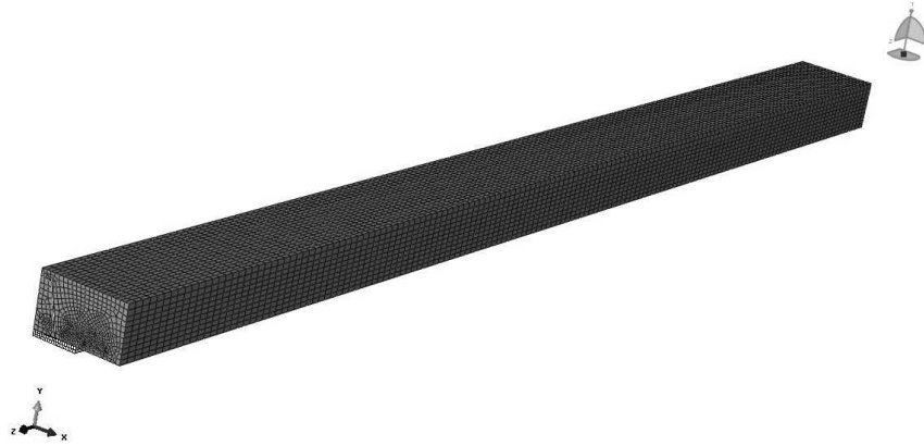
Fig. 3. 3D finite element model generated for the coupled thermal-structural analysis of DELTA composite beams.
