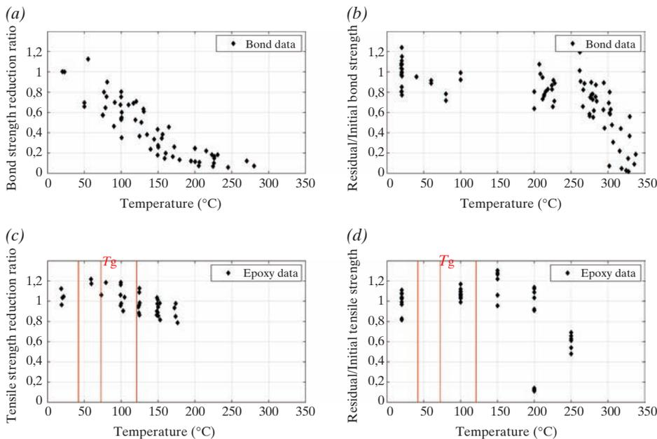
Fig. 3: Variation of (a) bond strength and (b) residual bond strength of FRPs and concrete with temperature and variation of (c) tensile strength and (d) residual tensile strength of epoxies with temperature
