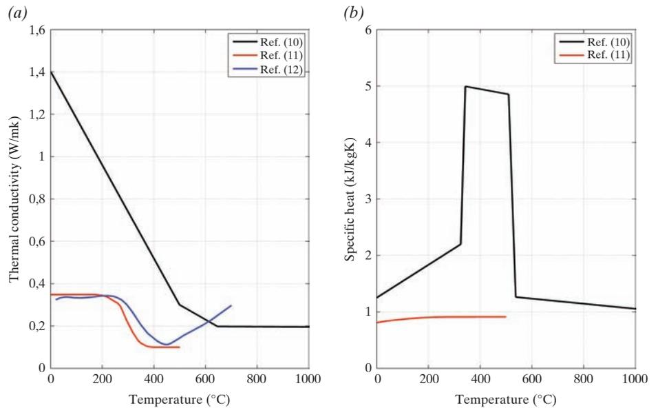
Fig. 1: Variation of (a) thermal conductivity and (b) specific heat of FRP materials with temperature
