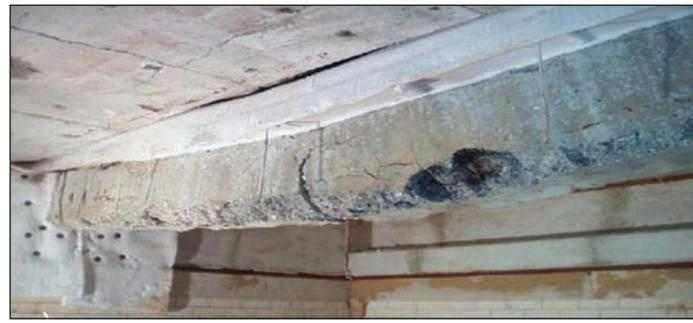
Fig. 7: Failure of FRP-reinforced beam<sup>34</sup>
