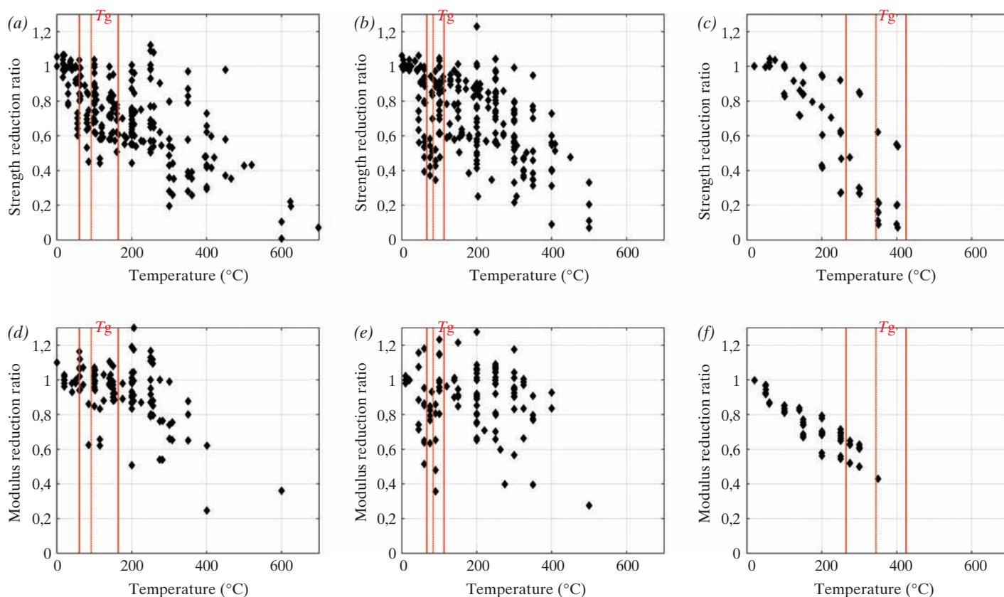
*Fig. 2: Variation of (a) CFRP, (b) GFRP and (c) AFRP ultimate tensile strength with temperature and variation of (d) CFRP, (e) GFRP and (f) AFRP modulus of elasticity with temperature*
