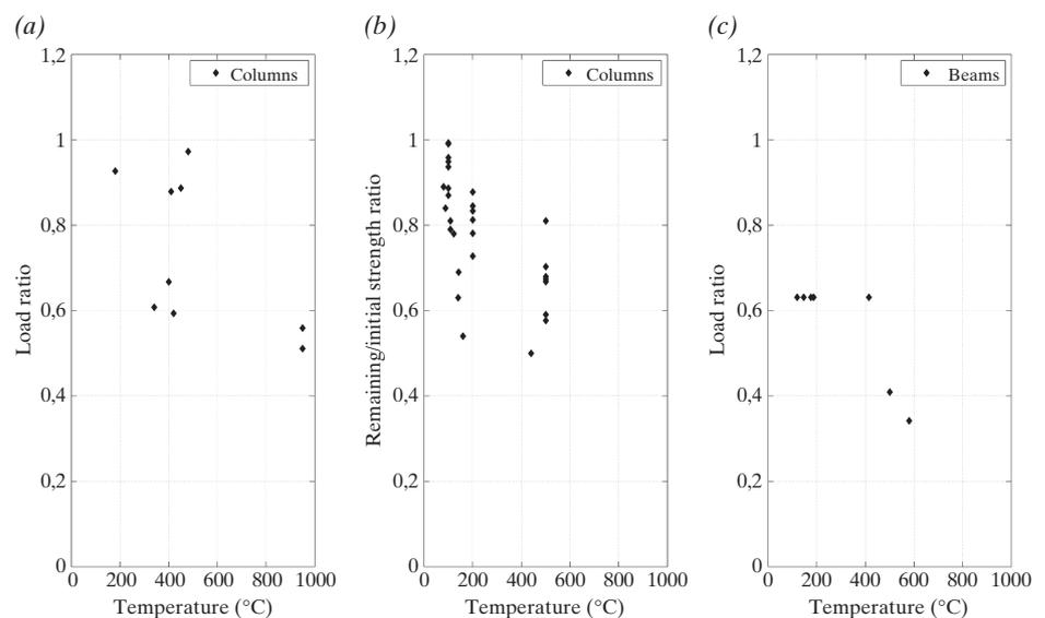
Fig. 8: Plot of (a) load ratio of tested FRP-strengthened columns versus failure temperature, (b) ratio of residual by initial strength of tested FRP-strengthened columns versus maximum temperature during heating and (c) load ratio of tested FRP-strengthened beams versus failure temperature
