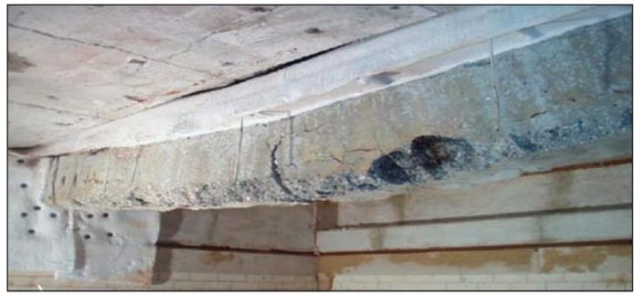
Fig. 7: Failure of FRP-reinforced beam<sup>34</sup>
