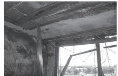
Fig. 10: View of the compartment after one of the Dalmarnock fire tests<sup>68</sup>
