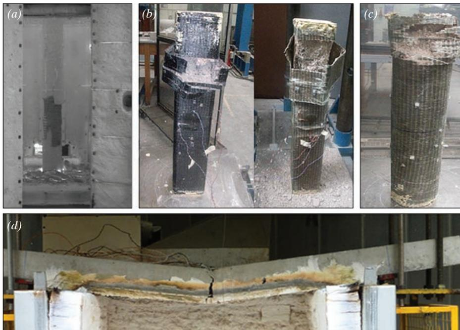
Fig. 9: Failure of (a) FRP-reinforced column,<sup>59</sup> (b) rectangular column with FRP wrap,<sup>60</sup> (c) circular column with FRP wrap<sup>61</sup> and (d) FRP-strengthened beam<sup>41</sup>
